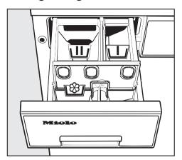
= Compartment for pre-wash. This compartment is also used for starch formulations when starching separately.
